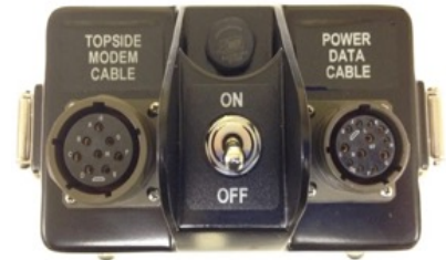
Figure 10: Topside Battery Unit Connections
